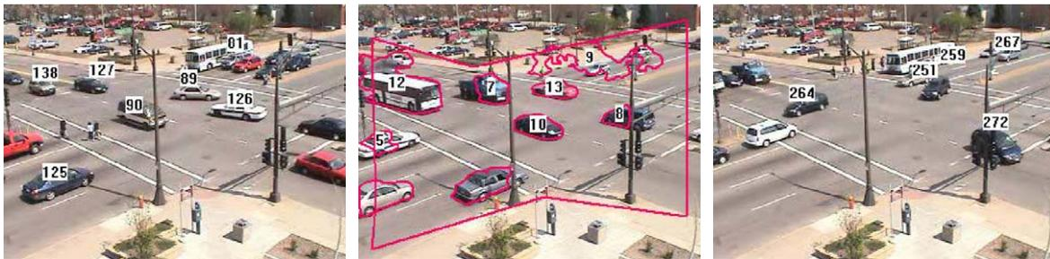
Fig. 9. Scene II: tracking vehicles in crowded scenes. The contours correspond to the blobs detected around the vehicles. Some of the contours are larger due to oversegmentation resulting from an illumination change.
