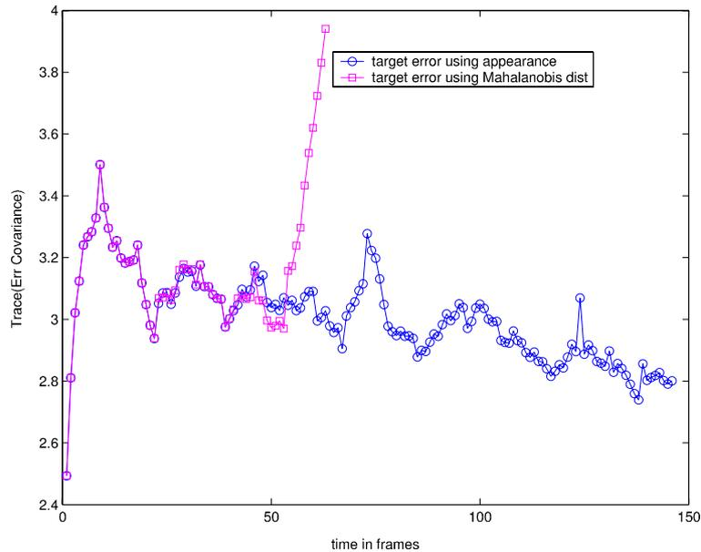
Fig. 15. Tracking errors for feature tracking using the Mahalanobis distance and geometric template constrained data association. The increase in error for the Mahalanobis distance constrained feature tracker after frame 40 is the result of the tracker switching to another target during an occlusion.
