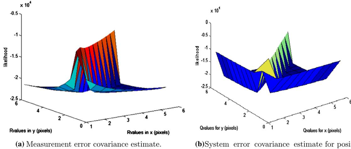
Fig. 3. Log likelihood estimates of measurement error. The surface plots correspond to the log likelihood of the errors in  $(x, y)$  positions for the measurement and system error expressed in the image coordinates, obtained at the end of EM procedure.  $x$ - and  $y$ -axis correspond to the error in  $x$  and  $y$  coordinates (in pixels), while the  $z$ -axis corresponds to the log likelihood obtained in the E step.
