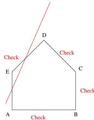
**Figure 9.** Checks that the segment intersection will perform.
