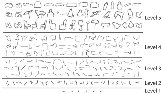
Figure 5. A. Examples of the mean shapes of visual concepts automatically learned for multiple objects with part sharing between objects (Zhu, Chen, Torralba, et al., 2011; Zhu, Chen, & Yuille, 2011). The specificity and the number of types of features increases as one goes up the hierarchy, consistent in general terms, with the progression of neural selectivities as one moves up the ventral stream.
