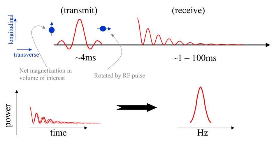
Signal acquired in time domain is transformed to frequency domain
