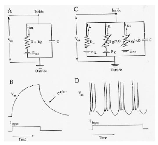
From Segev (1992). A. illustrates an RC-circuit at a single point of *passive* membrane. B is the temporal response to a step current input. C illustrates additional variable conductance components that model the electrical processes of spike generation (panel D)--the *active* properties. To model the active properties, one needs a more complicated set of differential equations: the Hodgkin-Huxley equations. (See Claude Meunier and Idan Segev, 2002 for an overview and recent critique).
