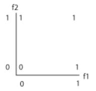
Make a similar truth table for XOR. Plot the logical outputs for the four possible input states. Can you draw a straight line to separate the 1's from the 0's?
