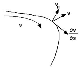
To make the problem well-posed, smoothness is imposed by requiring that a measure of the magnitude of the rate of change of the contour velocity along the contour, e.g.  $|\partial v/\partial s|^2$  be small.
