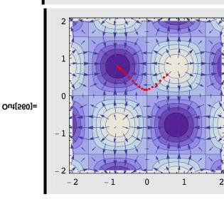
result = NestList[newr, {u0, v0}, 200]; In[558]:= gresults = ListPlot[result, PlotJoined->False, AxesOrigin->{0,0}, PlotRange->{{-2,2},{-2,2}},FrameLabel->{"u","v"}, Frame->True, AspectRatio->1, RotateLabel->False, PlotLabel->"State Space" Ticks->None, PlotStyle->{RGBColor[1,0,0], PointSize[0.015]}];
