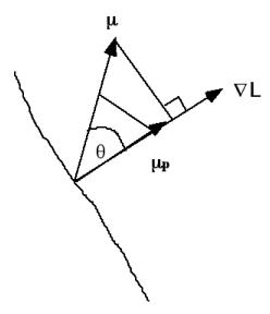
This formula makes explicit what we get, and what we lack in our effort to find a unique solution to the optic flow. We can get the velocity components in the direction of the gradient at each point, but not perpendicular to it. This ambiguity is known as the aperture problem. This problem is faced by any purely local measurements of motion. For example, the motion and orientation selective cells in V1, are limited by the aperture problem because of their small, limited receptive field sizes.
