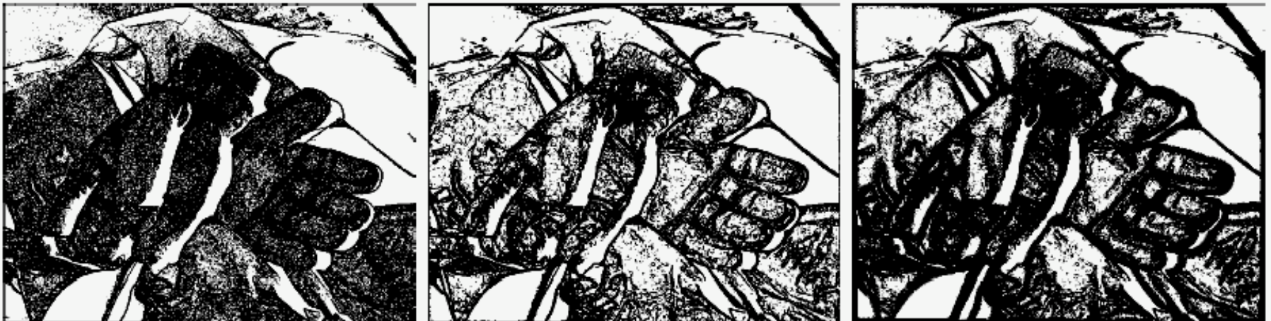
Figure 2.6 The edge estimated on the glove image by ML with the filter at scale 0 (left), filter at scale 1 (centre), and filter with scales 0, 1, 2, 4 (right). Observe that ML significantly overestimates the number of edges in this image.
