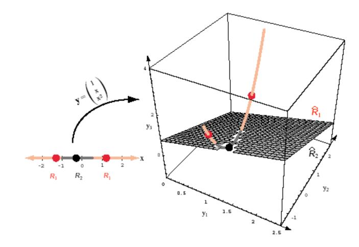
Figure 5.5: The mapping  $\mathbf{y} = (1, x, x^2)^t$  takes a line and transforms it to a parabola in three dimensions. A plane splits the resulting  $\mathbf{y}$  space into regions corresponding to two categories, and this in turn gives a non-simply connected decision region in the one-dimensional x space.
